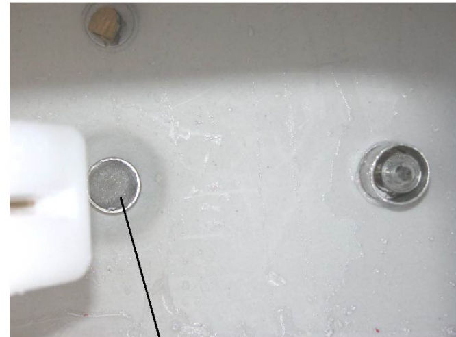
make sure pump filter install in solution tank all time to protect from damaging pump
