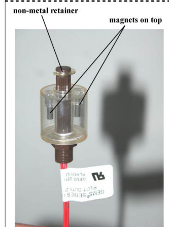
WRONG position of level switch
